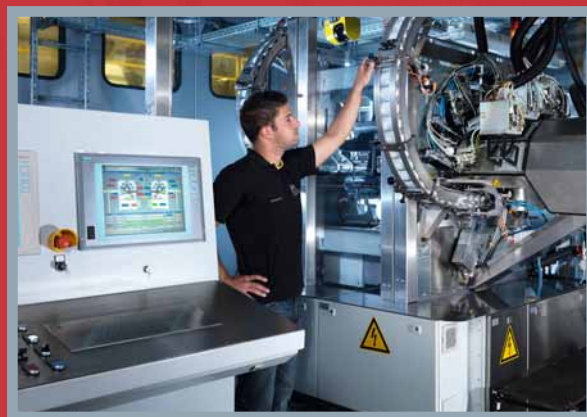
The prototype digital printing press at Ball Packaging Europe's Hassloch plant prints 120 cans a minute in normal production.
